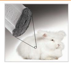
The continuous spinning of angora rabbit wool-like fibers from a non-equilibrated gelatin/water/2-propanol mixture using the presented process allows the production of protein fibers with simultaneous high porosity and promising mechanical properties.
