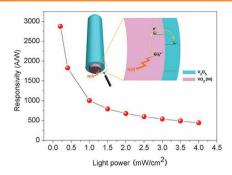
First oxide-catalogue photoconductive NIR detector built by the inner single-domain monoclinic VO<sub>2</sub> (M) core and outer V<sub>2</sub>O<sub>5</sub> shell is put forward, which accomplished an ultrahigh responsivity  $(R_{\lambda})$  of 2873.7 A W<sup>-1</sup> and specific detectivity (D\*) of  $9.23 \times 10^{12}$  Jones at room temperature (at 990 nm; 0.2 mW cm<sup>-2</sup>), recording the best performance compared with those reported IR detectors based on heavymetal-free materials.
