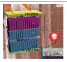
A novel stack-integrated photo-supercapacitor (PSC) thin-film device is composed of a dye-sensitized solar cell and a supercapacitor built on bi-polar anodic titanium oxide nanotube arrays. Improved supercapacitor performance is achieved through selective plasma-assisted hydrogenation treatment. A remarkable overall photoelectric conversion and storage efficiency up to 1.64% is achieved with a fast response and superior cycling capability.
