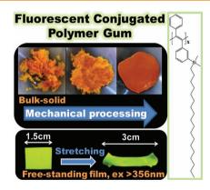
Long alkyl chain-coupled PDPA derivatives provide quite soft and sticky gums at room temperature to produce films with very smooth surfaces after manual kneading and pressing. The fluorescence emission is quite intense in both the film and solution. The elastomer-supported film accommodates the large strain without cracking and delamination, after stretching and relaxing several hundred times.
